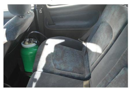
Fig. 4. New connected fuel tank
