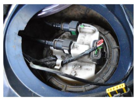
Fig. 1. In tank fuel pump
