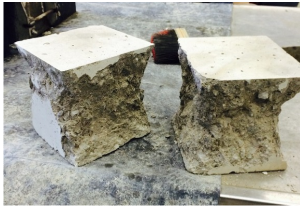
Fig. 14. The failure modes of compressive strength test specimens
