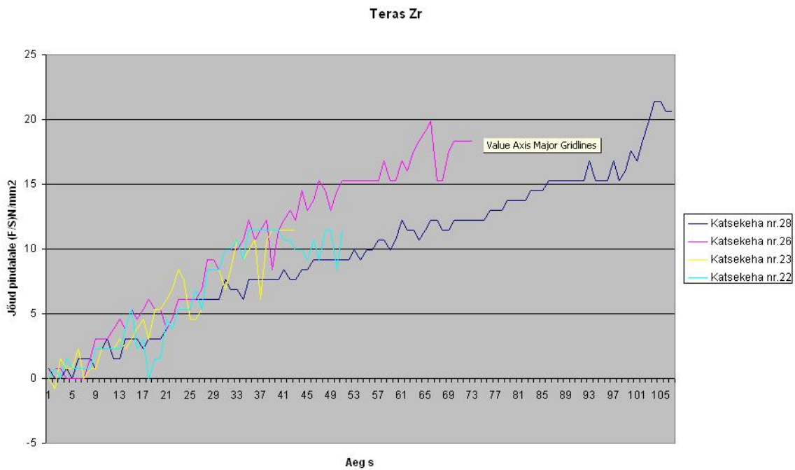
Fig. 11. The bond strength of coating ZrO_2/30CaO on steel
